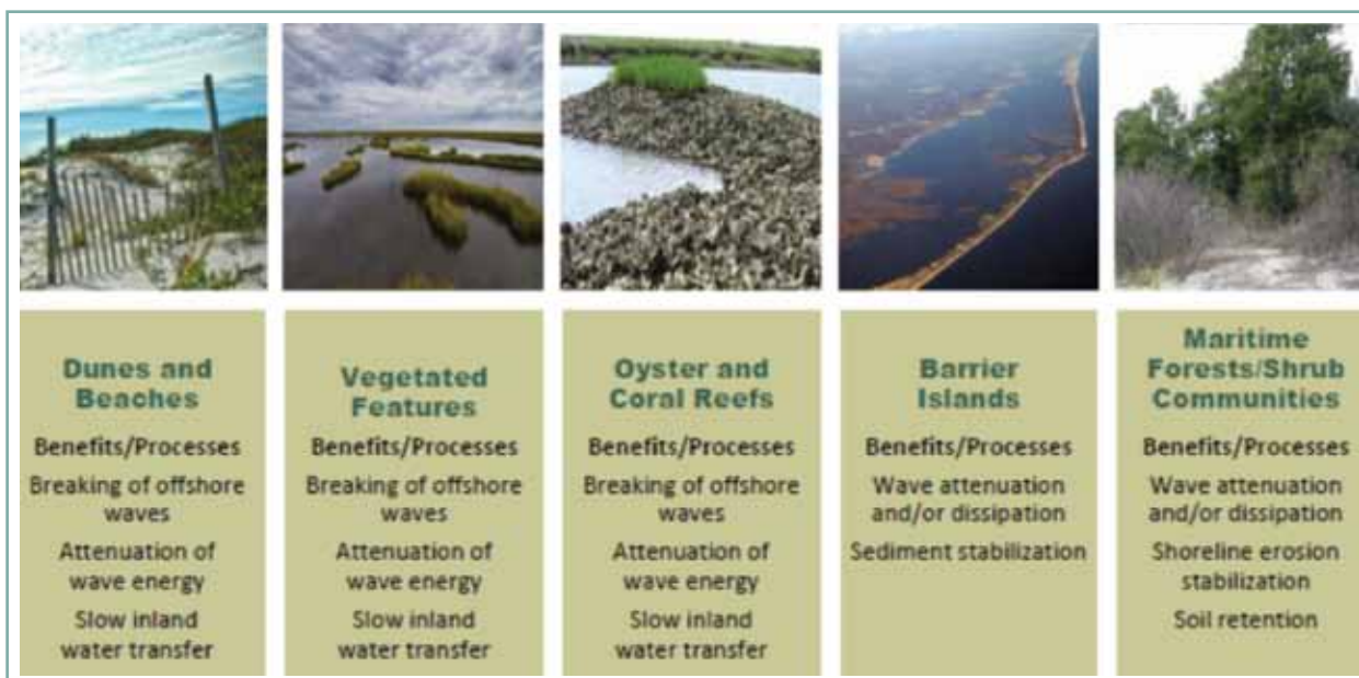
Figure 1. Natural and nature-based features at a glance. Adapted from: USACE. 2013. Coastal Risk Reduction and Resilience . CWTS 2013-3. U.S. Army Corps of Engineers, Washington, D.C.
