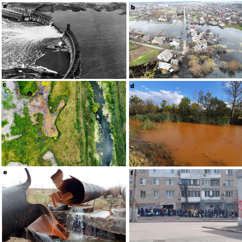
Fig. 3 | Examples of impacts on water resources and infrastructure in Ukraine during armed conflicts. a , The dam on the Dnieper River near the city of Zaporizhzhia after reportedly being blown up by Soviet special forces in 1941 in an attempt to delay the offence of German troops. b , Demolition of the dam on the Irpin River on 26 February 2022 caused flooding near the village of Demidov in the Vyshhorod district of Kyiv region. c , Craters formed by shells on the floodplain of the Irpin River. d , Water in the Kamyshevakha River polluted by
