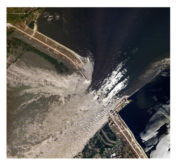
Figure 8. The destroyed Kakhovka facility on 6 June 2023 a few hours after the explosion (Source: https://twitter.com/GianlucaMezzo/status/1666097052269559816).
