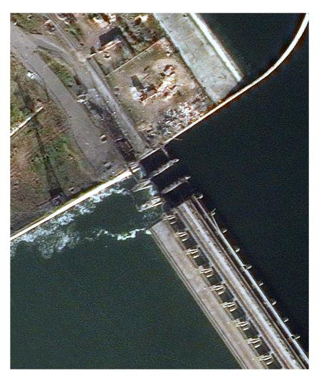
Figure 7. Satellite image of the damaged Kakhovka dam showing the damage to the roadway and dam on 11 November 2022 (Source: https://twitter.com/Maxar/status/1591158455808954368/photo/2).
